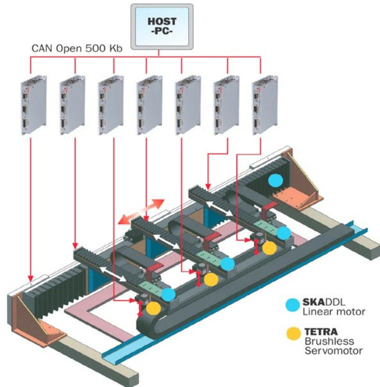
A Cello digital servo drive is connected to each axis on a Ceramic Tile Patterning Machine
