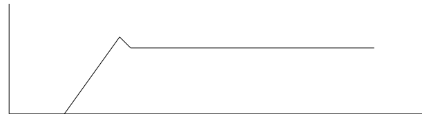
Critically damped: T5 optimum
