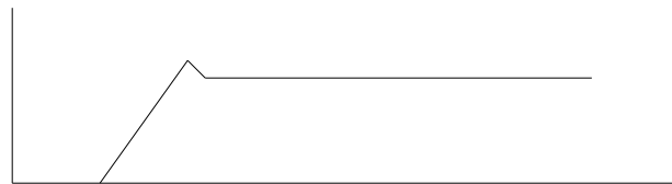
Critically damped: T1 optimum
