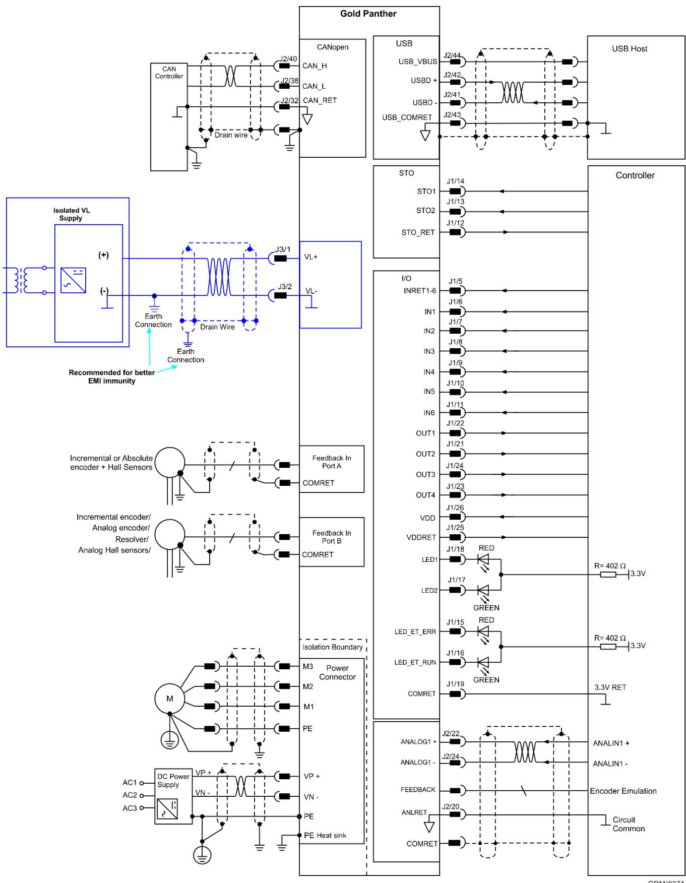
Figure 5: Gold Panther Connection Diagram for CAN – with Backup Functionality
