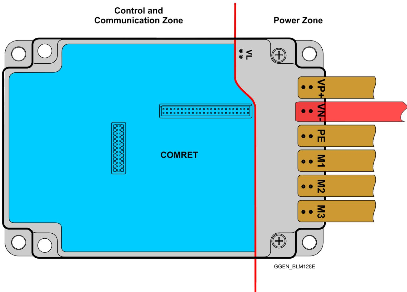
Figure 2: Gold Panther Power Conductors PCB layout
