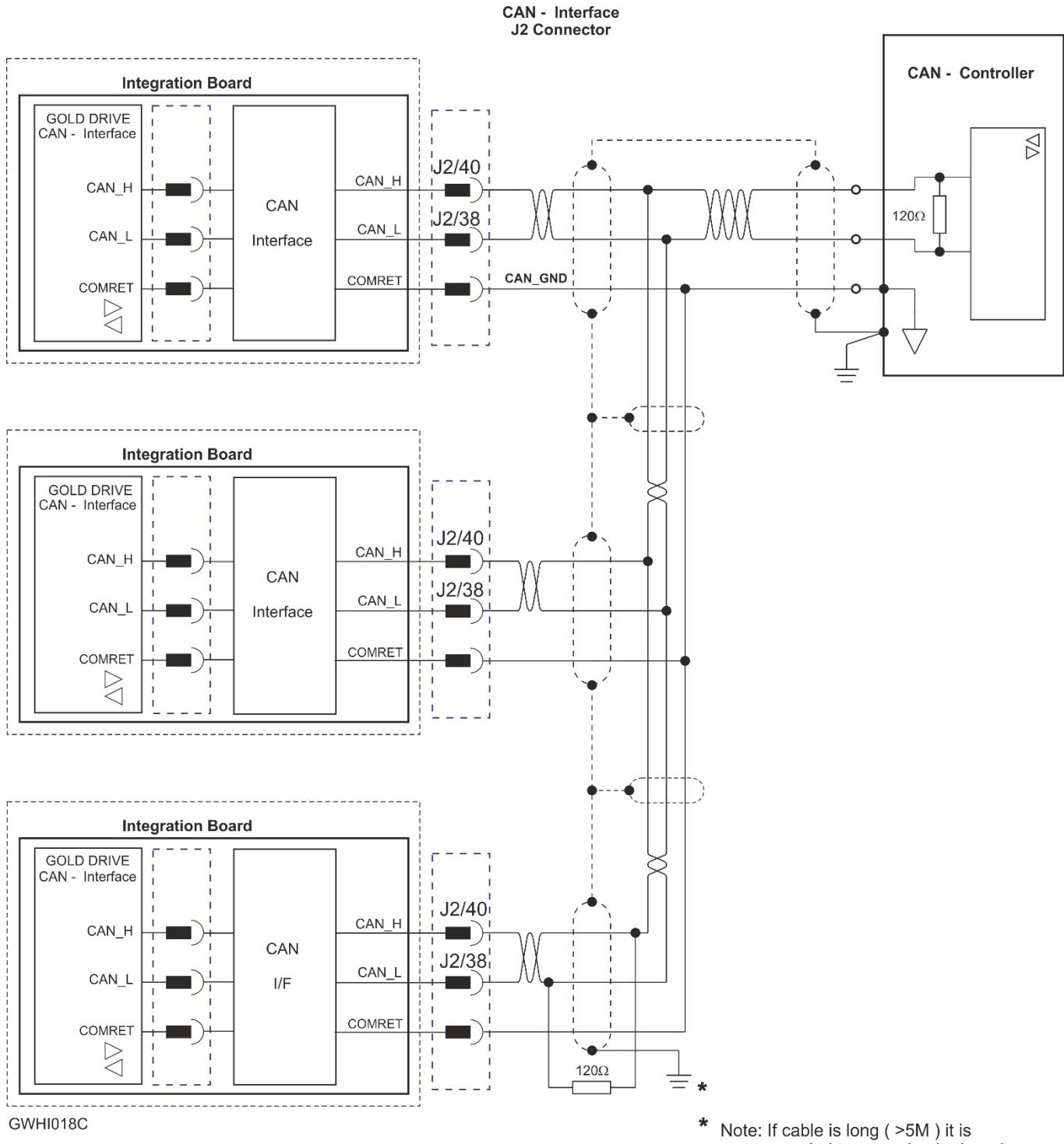
Figure 28: CANbus Connections
