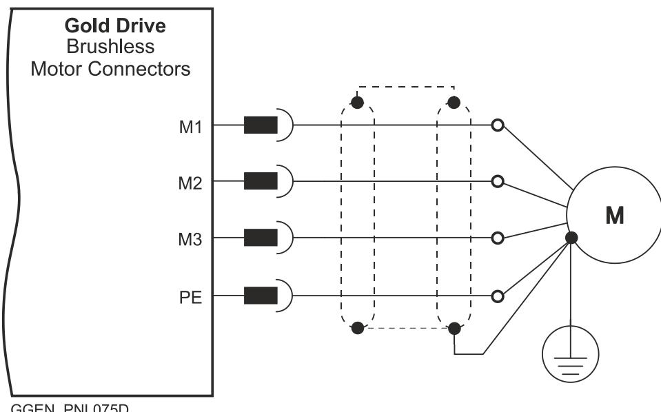
Figure 7: Brushless Motor Power Connection Diagram
