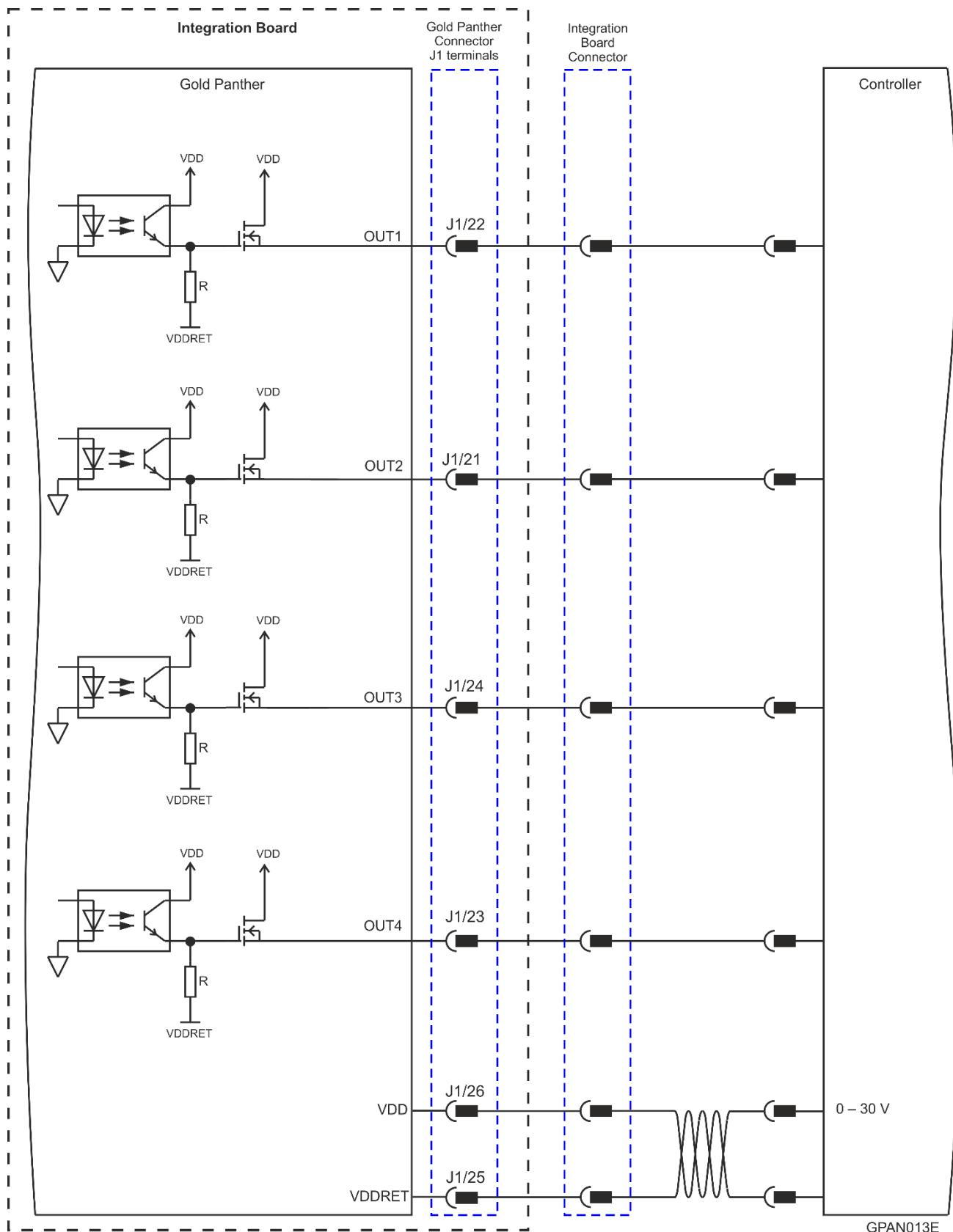
Figure 32: PLC Digital Output Connection Diagram For S or 0 Suffixes
