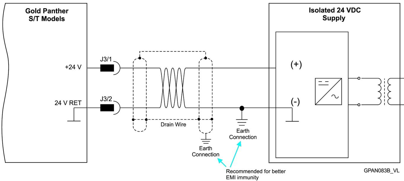
Figure 13: 24 VDC Control Supply Connection Diagram
