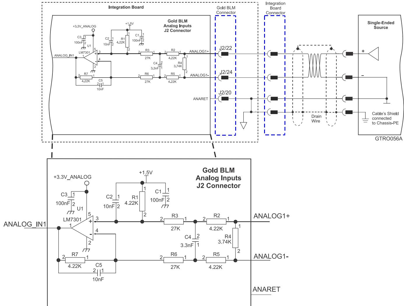
Figure 23: Analog Input with Differential  $\pm 10$  V
