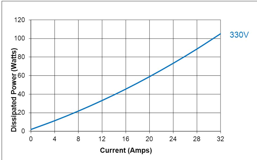
Figure 36: Dissipation versus Current Graph for 330 VDC
