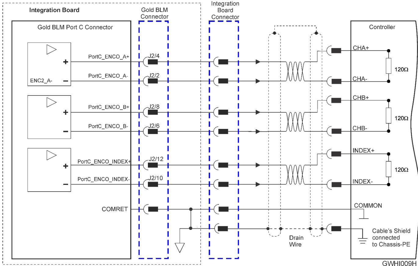
Figure 22: Emulated Encoder Differential Output – Recommended Connection Diagram
