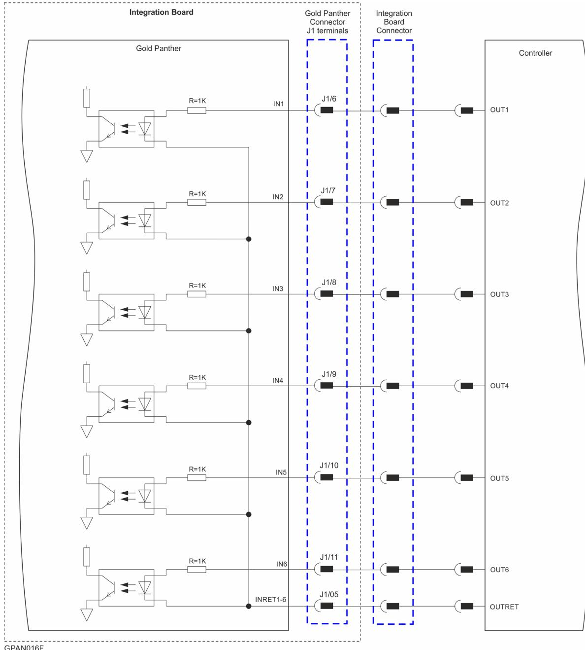
Figure 29: Digital Input TTL Mode Connection Diagram
