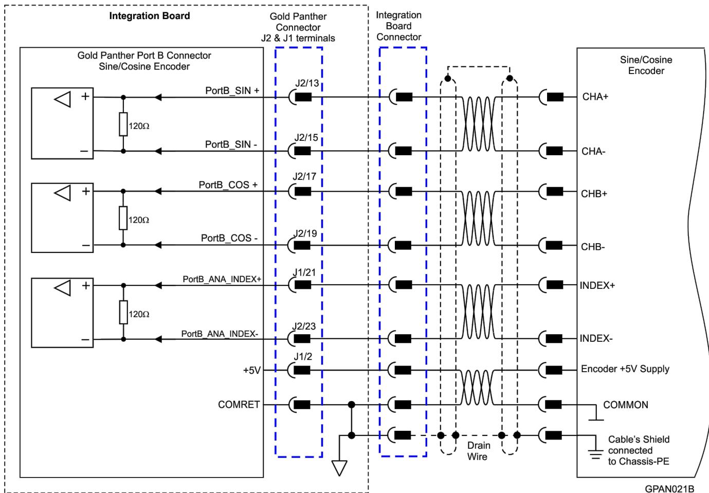
Figure 20: Port B - Interpolated Analog Encoder Connection Diagram
