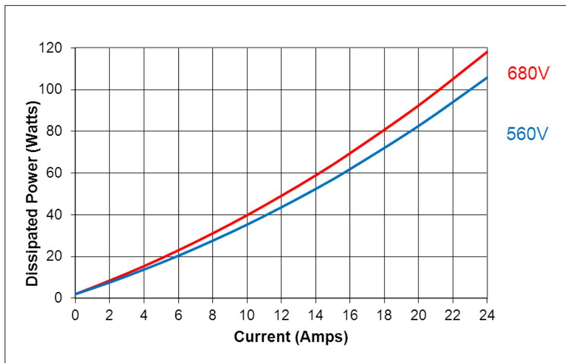
Figure 35: Dissipation versus Current Graph for 560 and 680 VDC
