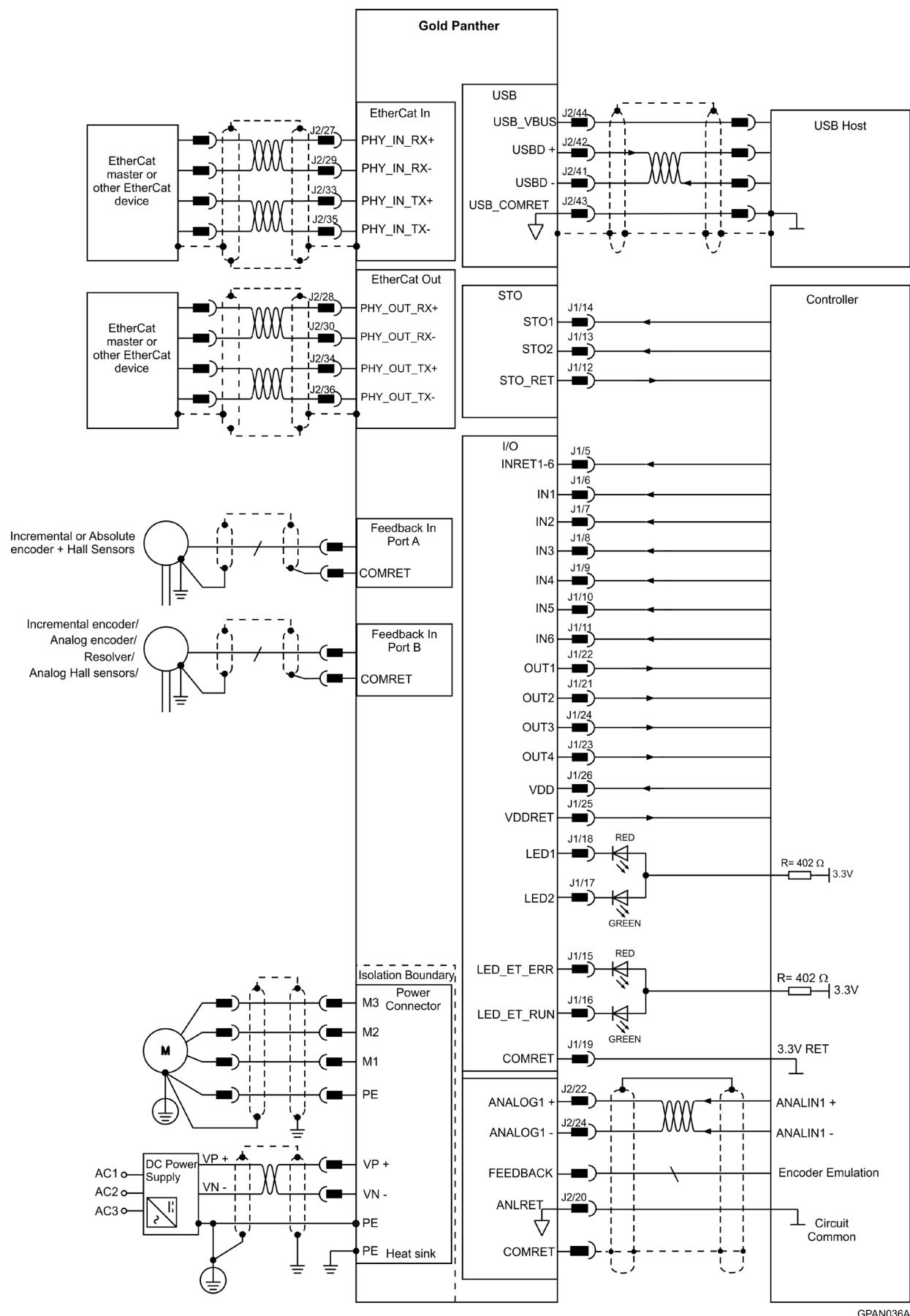
Figure 4: Gold Panther Connection Diagram for EtherCAT – 400 V without Backup Functions
