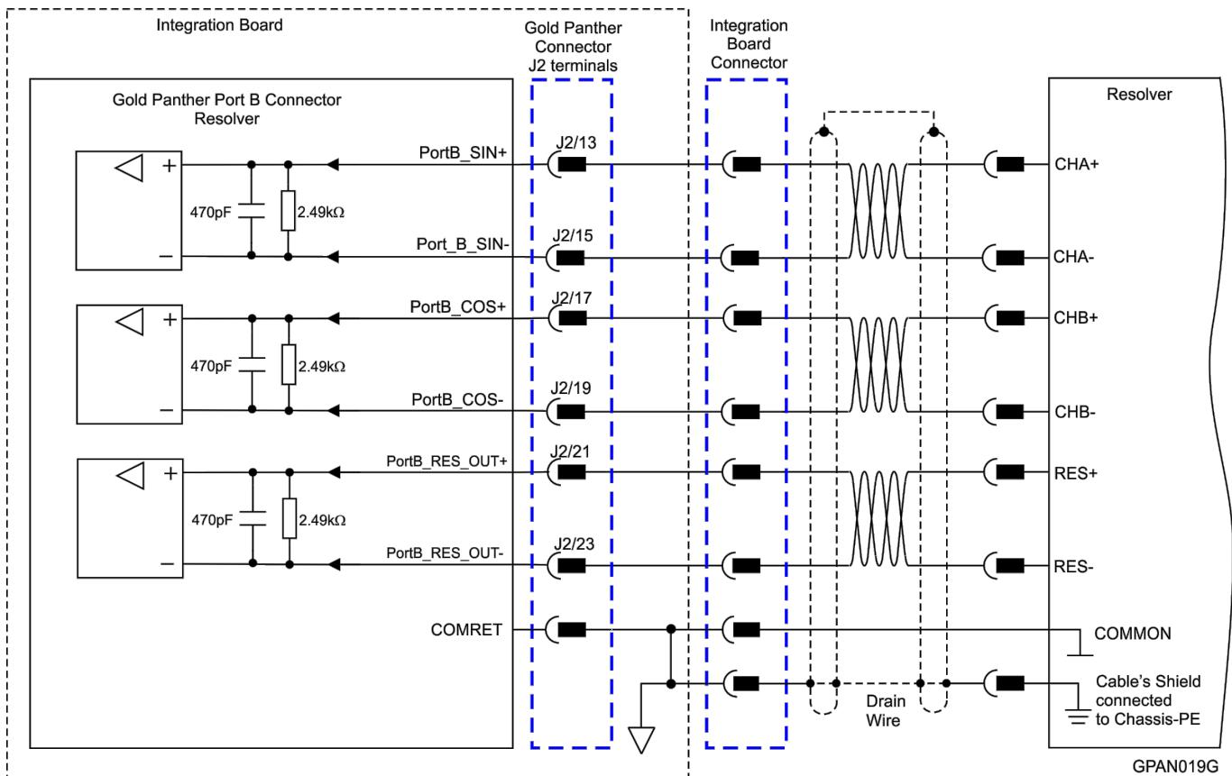
Figure 21: Port B – Resolver Connection Diagram
