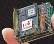
The Gold Bee is a tiny, highly intelligent, high-powered servo drive. Weighing only 20grams, the Gold Bee is the ideal servo drive to be "mounted anywhere". For example: Right on the motor, on moving axes or within robotic joints.
