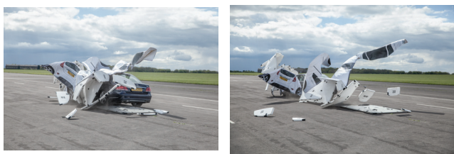
Figure 2: When the test vehicle collides with the GST, the foam of the Soft Car 360 flies apart harmlessly, leaving the test vehicle undamaged. (Courtesy of AB Dynamics)
