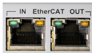
Figure 40: Ethernet Connector LEDs
